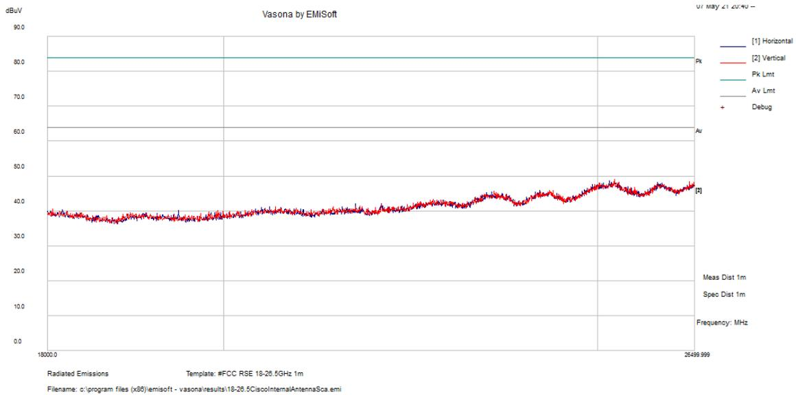
4) 26.5 - 40 GHz Scan, measured at 1 meter
