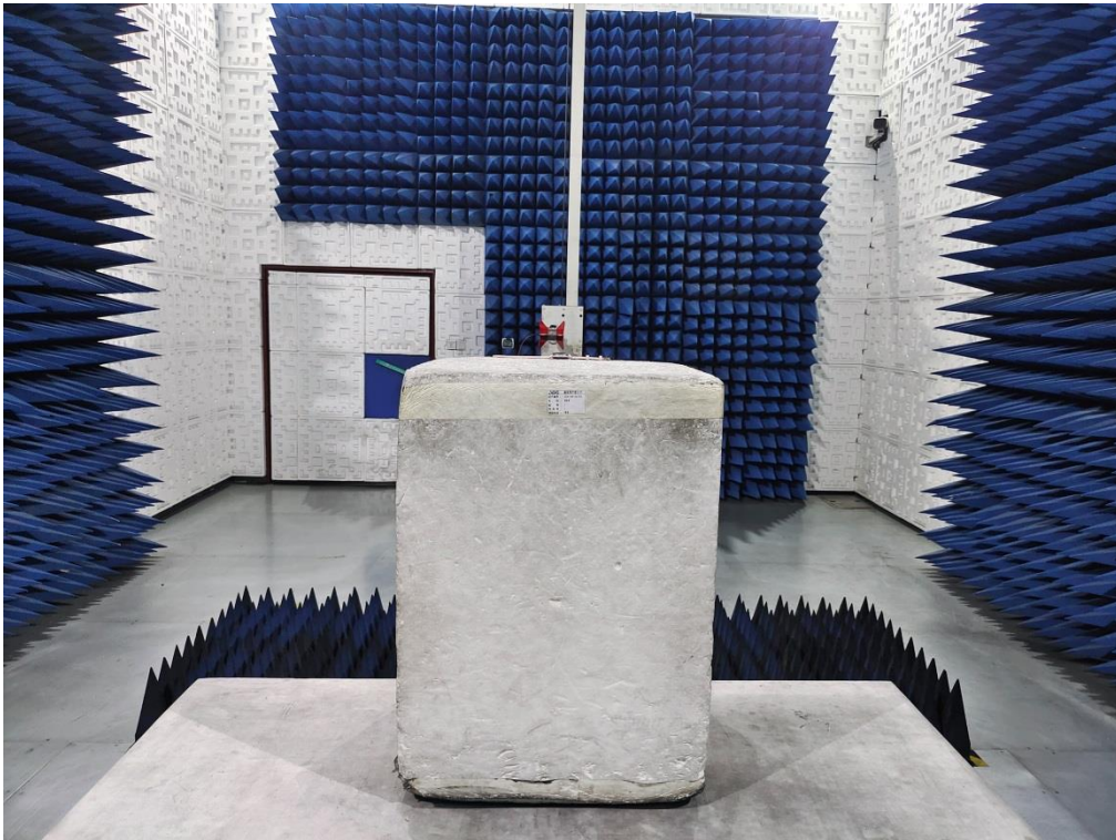
RADIATED EMISSION TEST SETUP ABOVE 1GHZ
