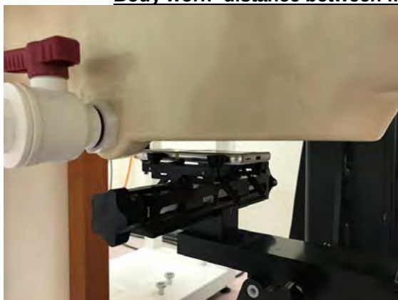
Fig.7 EUT Front side to flat phantom
