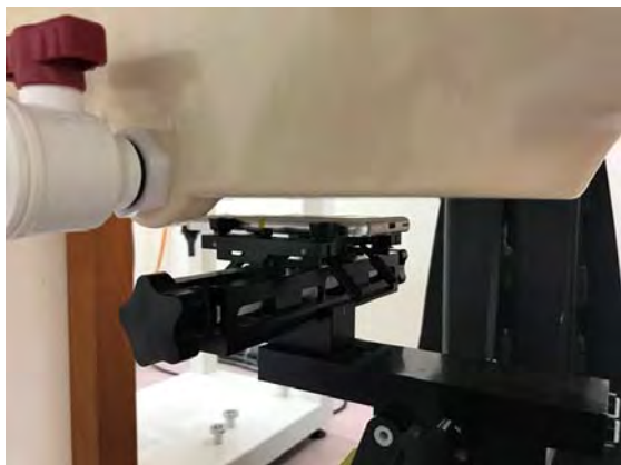
Fig.8 EUT Back side to flat phantom
