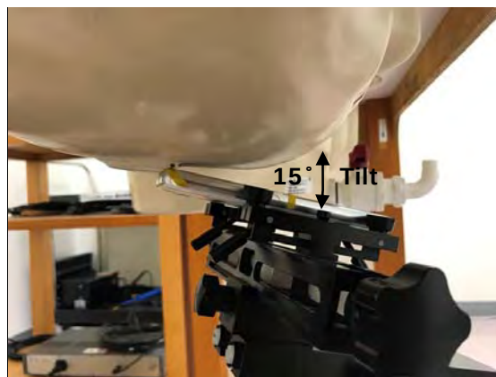
Fig.4 Right Head Section / Ear-Tilt Position(15°)
