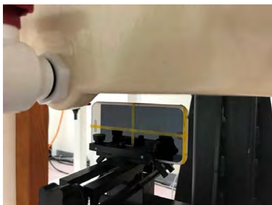
Fig.13 EUT Left side to flat phantom
