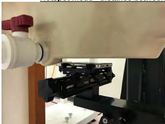
Fig.9 EUT Front side to flat phantom
