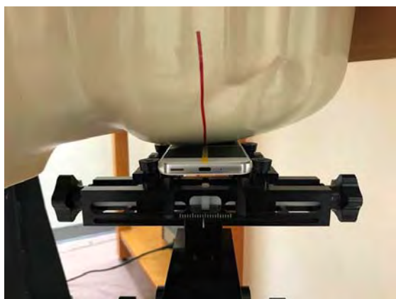
Fig.5 Left Head Section / Cheek-Touch Position
