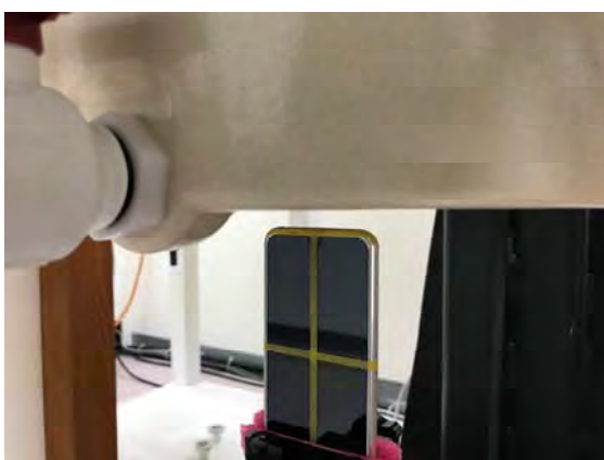
Fig.11 EUT Top side to flat phantom
