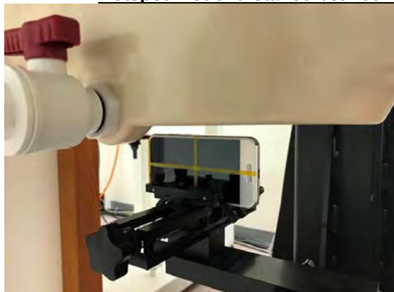
Fig.12 EUT Right side to flat phantom
