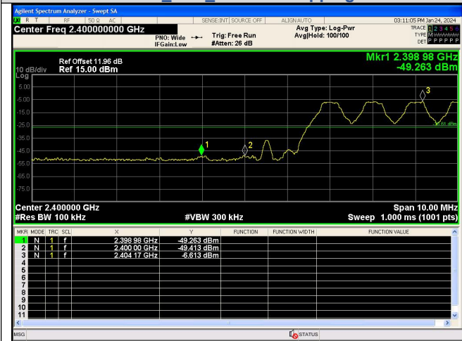
Out Of Band Emission(Left) GFSK_DH5_Channel Hopping
