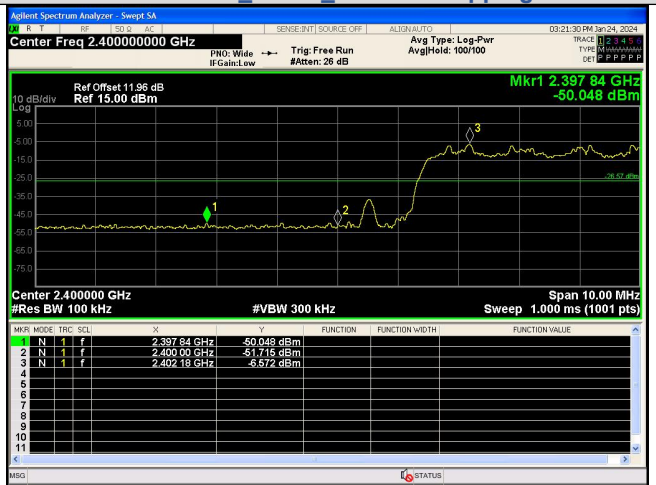
Out Of Band Emission(Left) \pi/4 DQPSK_2-DH5_Channel Hopping
