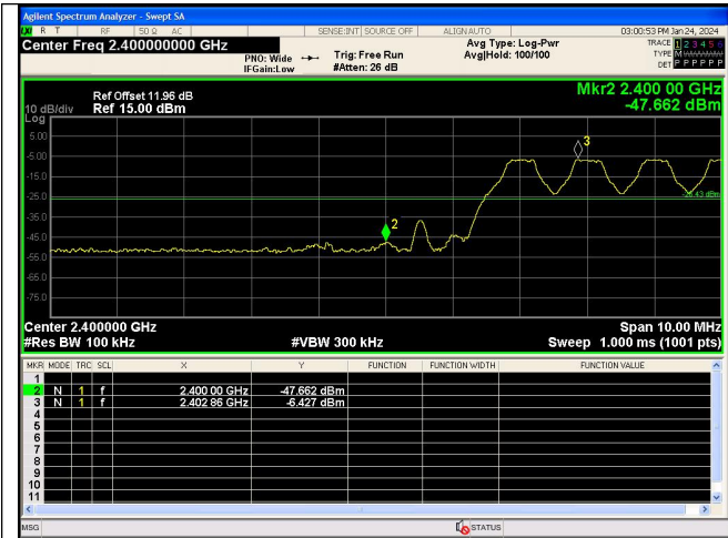
Out Of Band Emission(Left) GFSK_DH5_Channel Hopping
