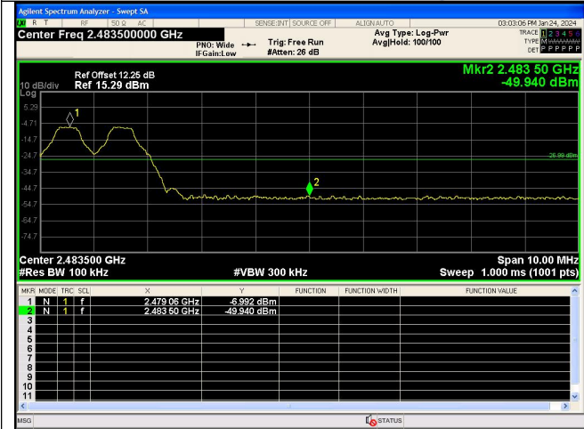
Out Of Band Emission(Right) GFSK_DH5_Channel Hopping
