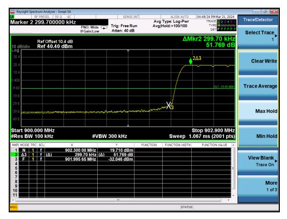
Screen Capture from the spectrum analyzer: Upper Band Edge (Hopping)
