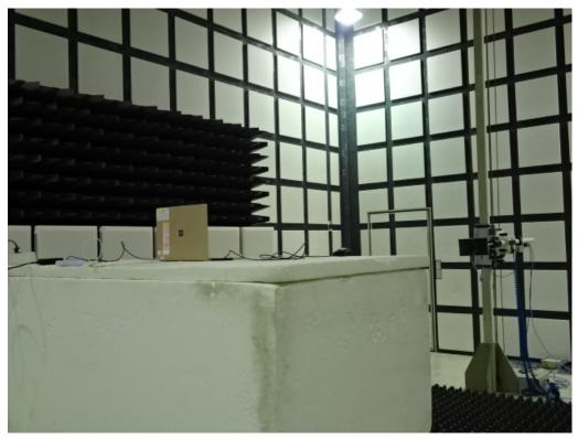
Radiated Emission Set up Photos (Above 18GHz)
