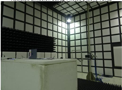
Radiated Emission Set up Photos (Above 18GHz)
