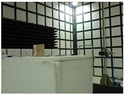
Radiated Emission Set up Photos (Above 18GHz)
