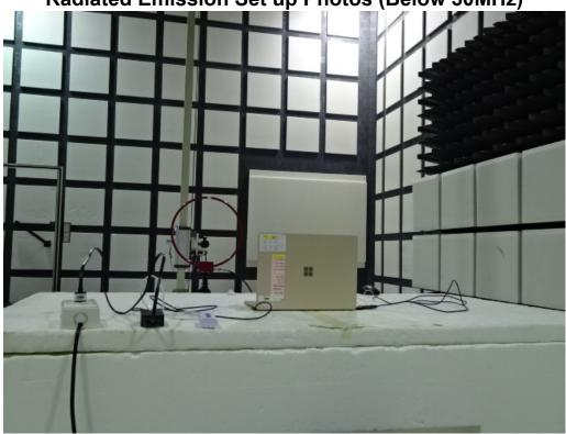
Radiated Emission Set up Photos (Below 1GHz)
