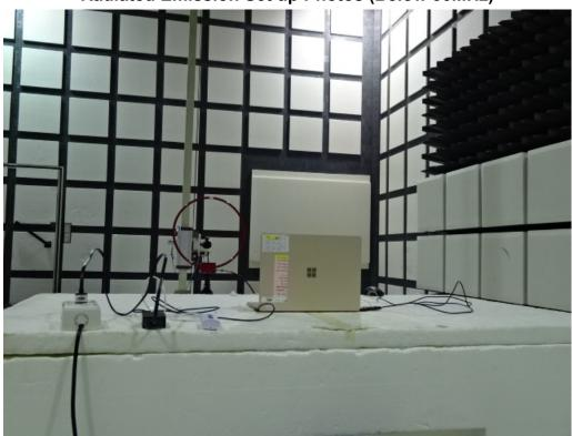
Radiated Emission Set up Photos (Below 1GHz)
