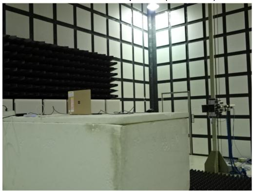
Radiated Emission Set up Photos (Above 18GHz)
