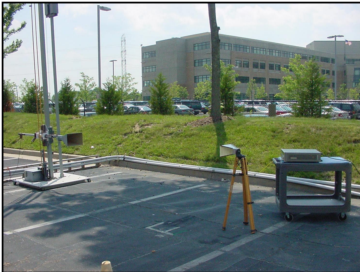
PHOTOGRAPH 4: SUBSTITUTION TRANSMITTING HORN ANTENNA 1-18GHZ
