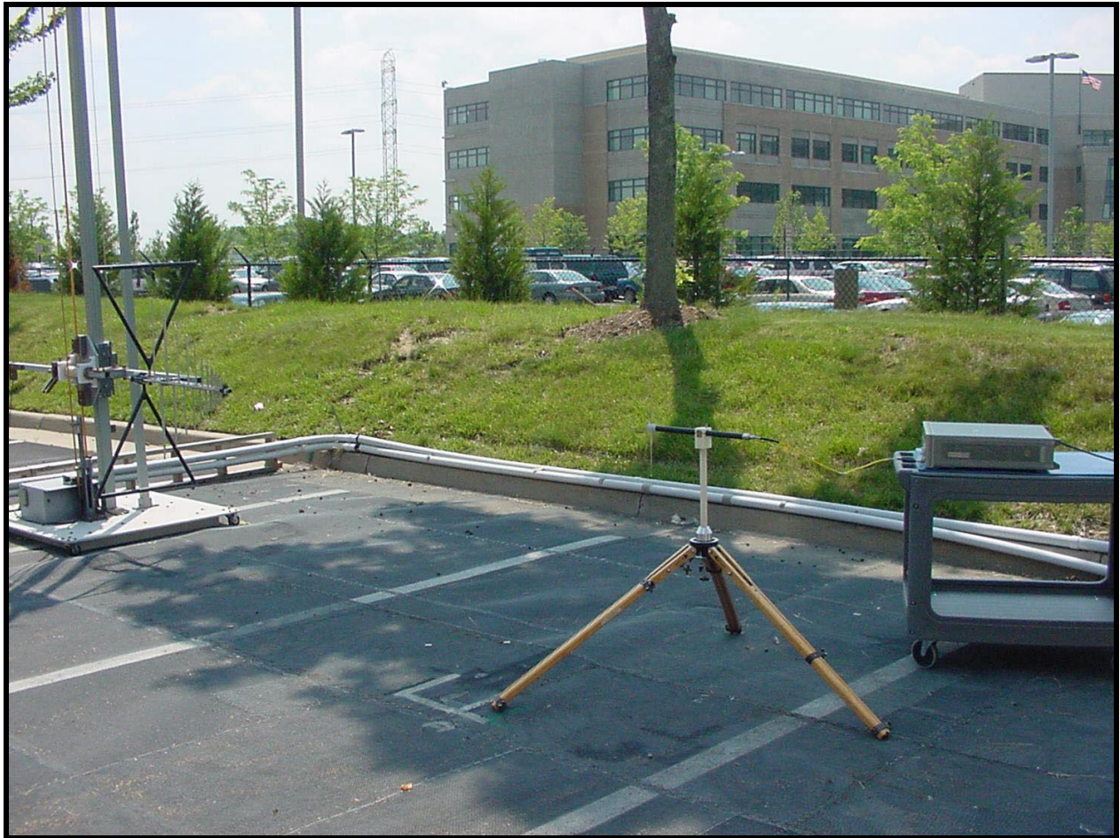
PHOTOGRAPH 5: SUBSTITUTION TRANSMITTING DIPOLE ANTENNA 30 MHZ - 1GHZ
