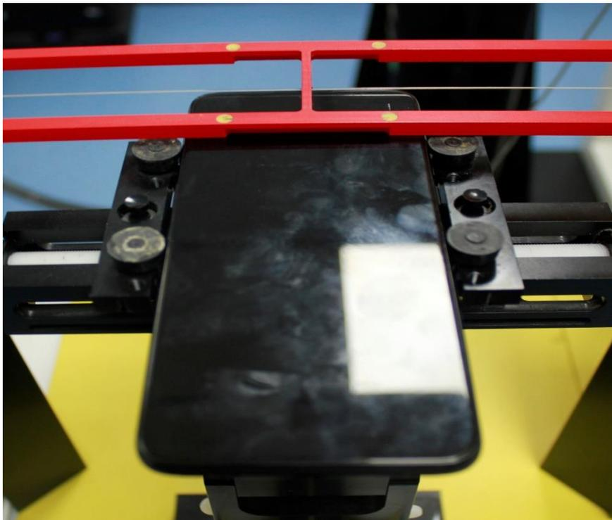
**Picture 2: EUT Positioning for RF**
