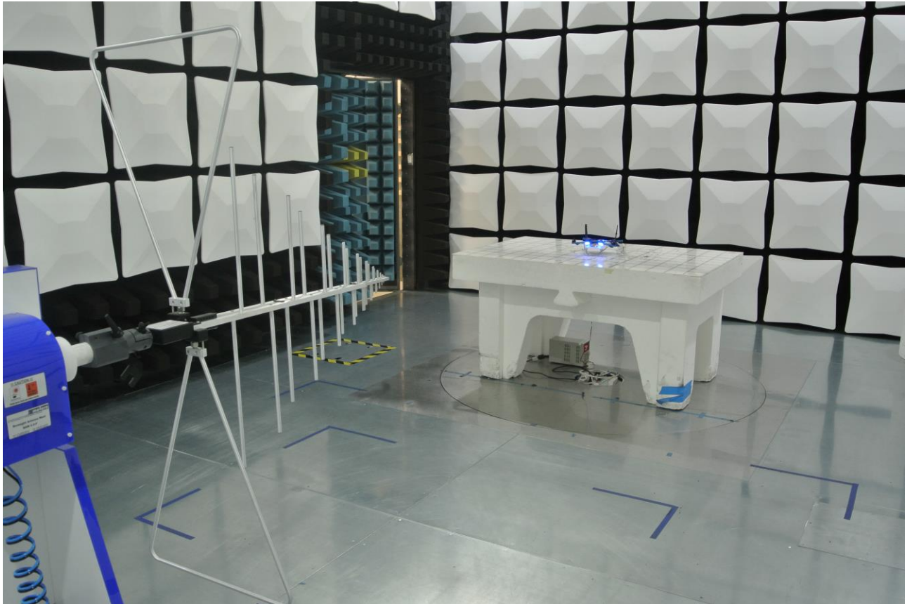
Figure 3: Test Setup for Radiated Emissions 30MHz to 1000MHz
