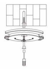
4. Align the notch on the bottom of the camera with the raised portion of the base and install the snap-fit, and then rotate the lock clockwise until it locks into place.
