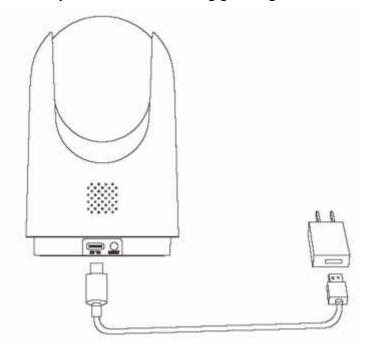
Tip: After turning on the camera, please do not twist the lens of the camera to force it to rotate. If the lens is not positioned accurately, it can be calibrated through the APP.
