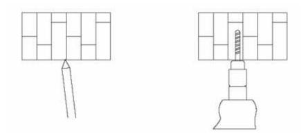
2. Screw the two plastic expansion nuts into the holes.
