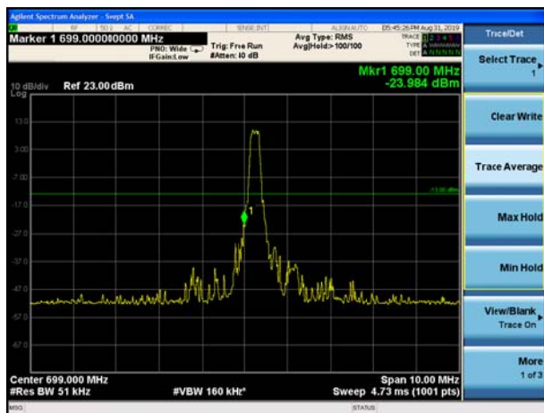
LTE Band 12 QPSK 1.4MHz CH-Low, 100%RB
