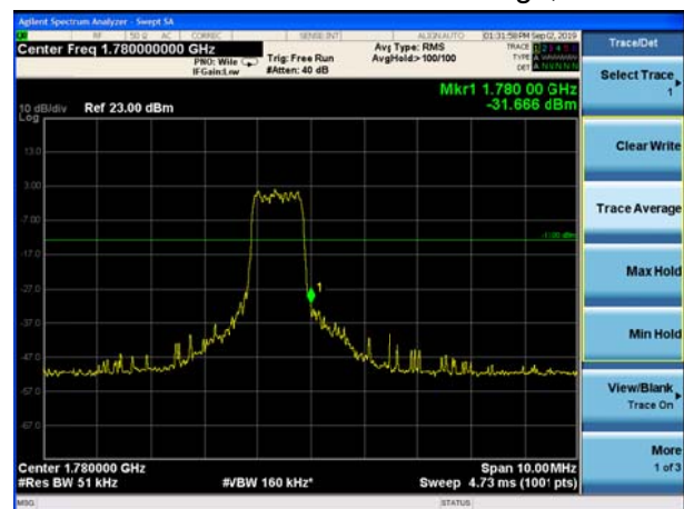
LTE Band 66 16QAM 3MHz CH-High, 1 RB
