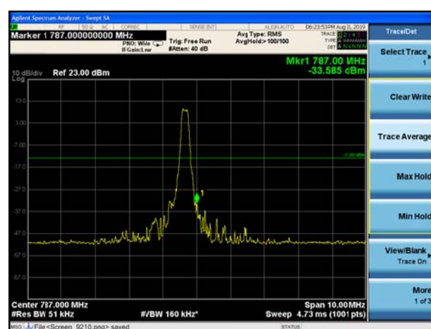
LTE Band 13 QPSK 5MHz CH- High, 100%RB
