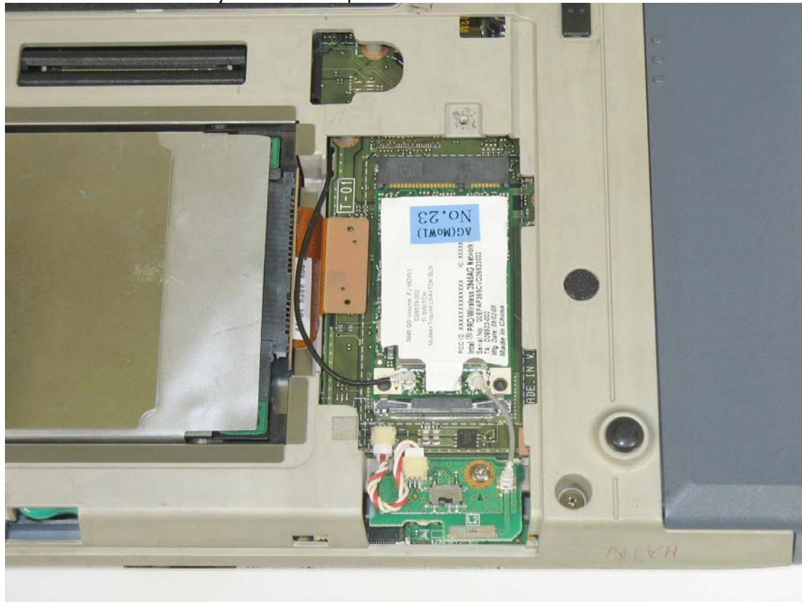
WM3945ABG inside the Fujitsu Tablet Computer
