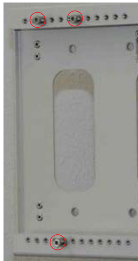
9764 Metro Dock attachment bolts on support plate
