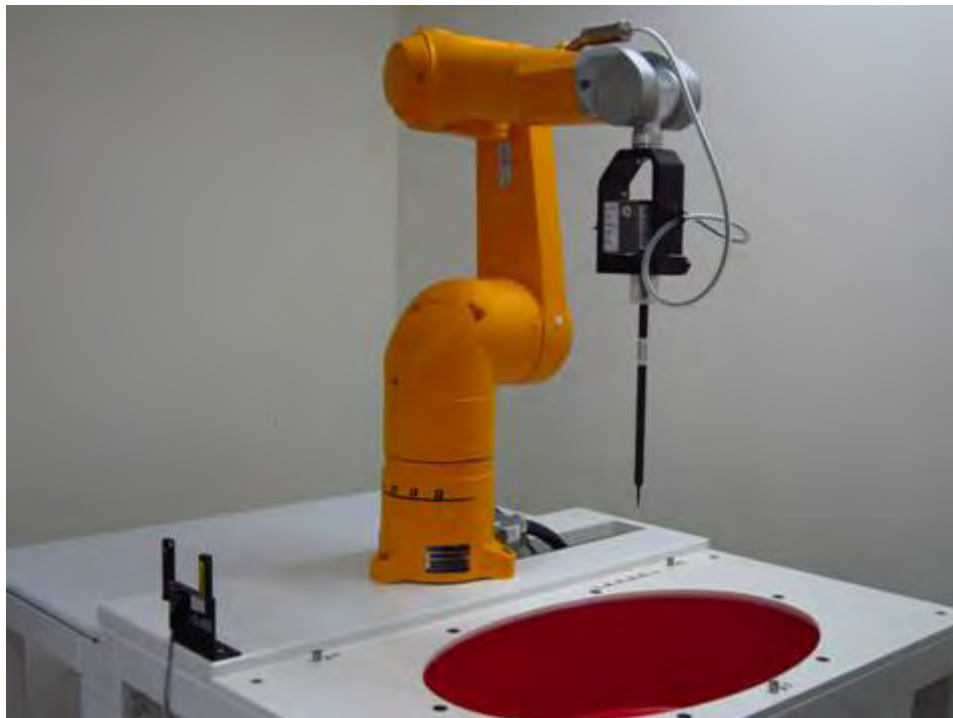
Fig.1 Photograph of the SAR measurement system
