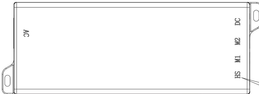
Insert the BTD02 to the HS plug of the control box
