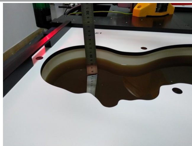
Liquid depth in the Head phantom
