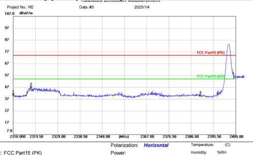
Limit: FCC Part15 (PK) EUT: Bluetooth module M/N: FSC-BT9104DI
