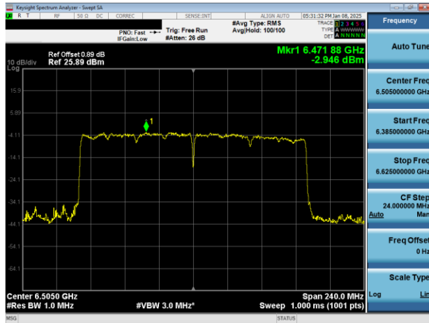
Plot 7-479. PSD Plot CDD Diversity Antenna 5T (160MHz 802.11ax RU996x2 (UNII Band 6) – Ch. 111)
