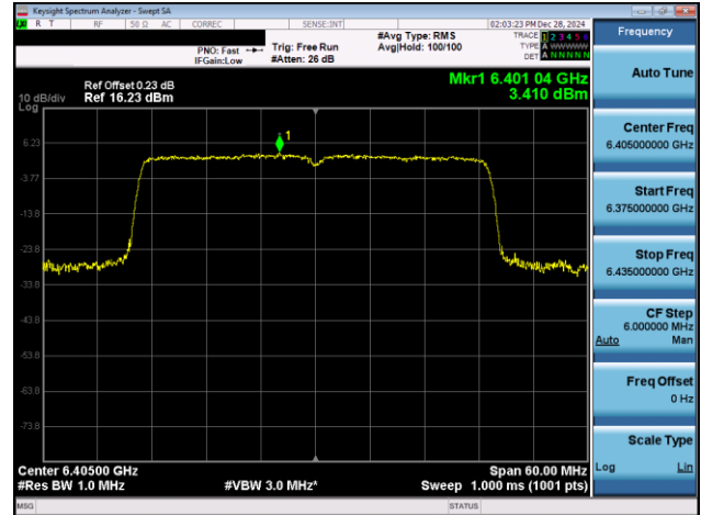
Plot 7-460. PSD Plot CDD Diversity Antenna 1b (40MHz 802.11ax RU484 (UNII Band 5) – Ch. 91)
