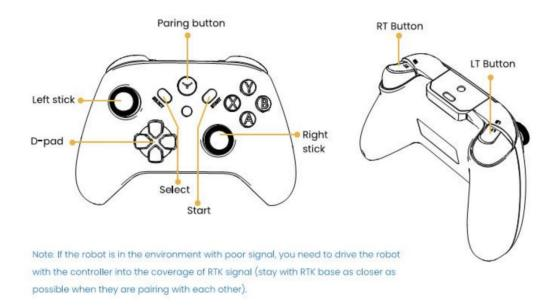
Paring button: Start to search and pair with the robot (Emergency stop button: pairing button can
