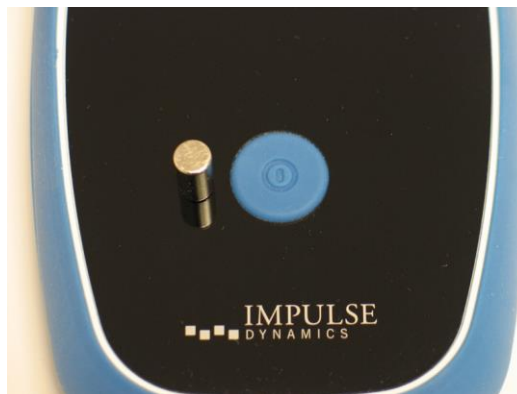
Figure 80: Pairing Magnet on Guardio Charger
