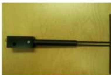
Figure 1 – MVG COMOSAR Validation Dipole
