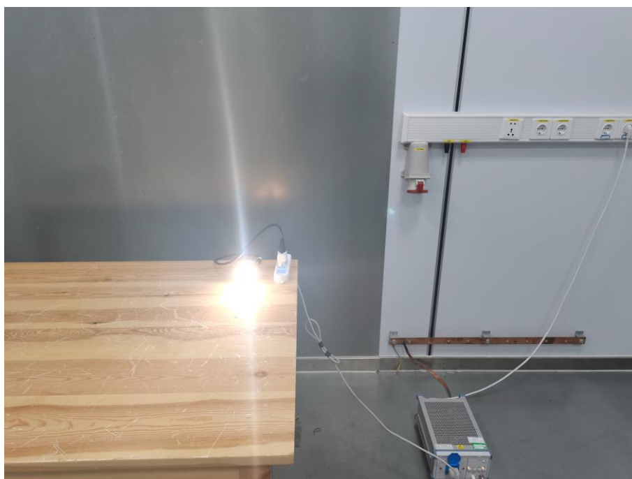
Fig. 4 Power line conducted emission setup photo
