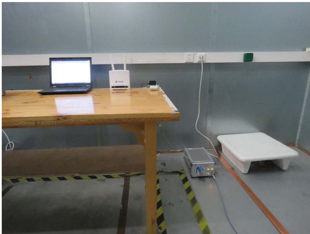
Picture 3 Conducted Emission Test Setup
