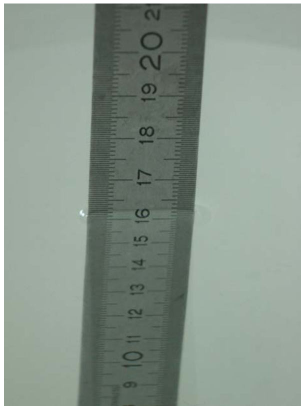
Fig. 26: Liquid depth for GPRS 1900 Body measurements.
