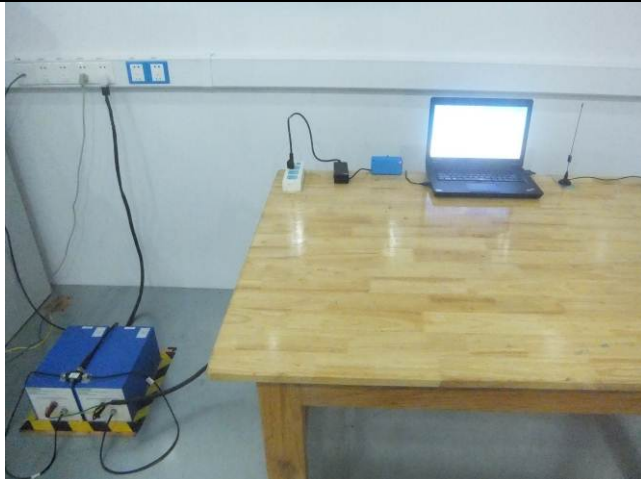
Conducted Emissions Test Setup Front View
