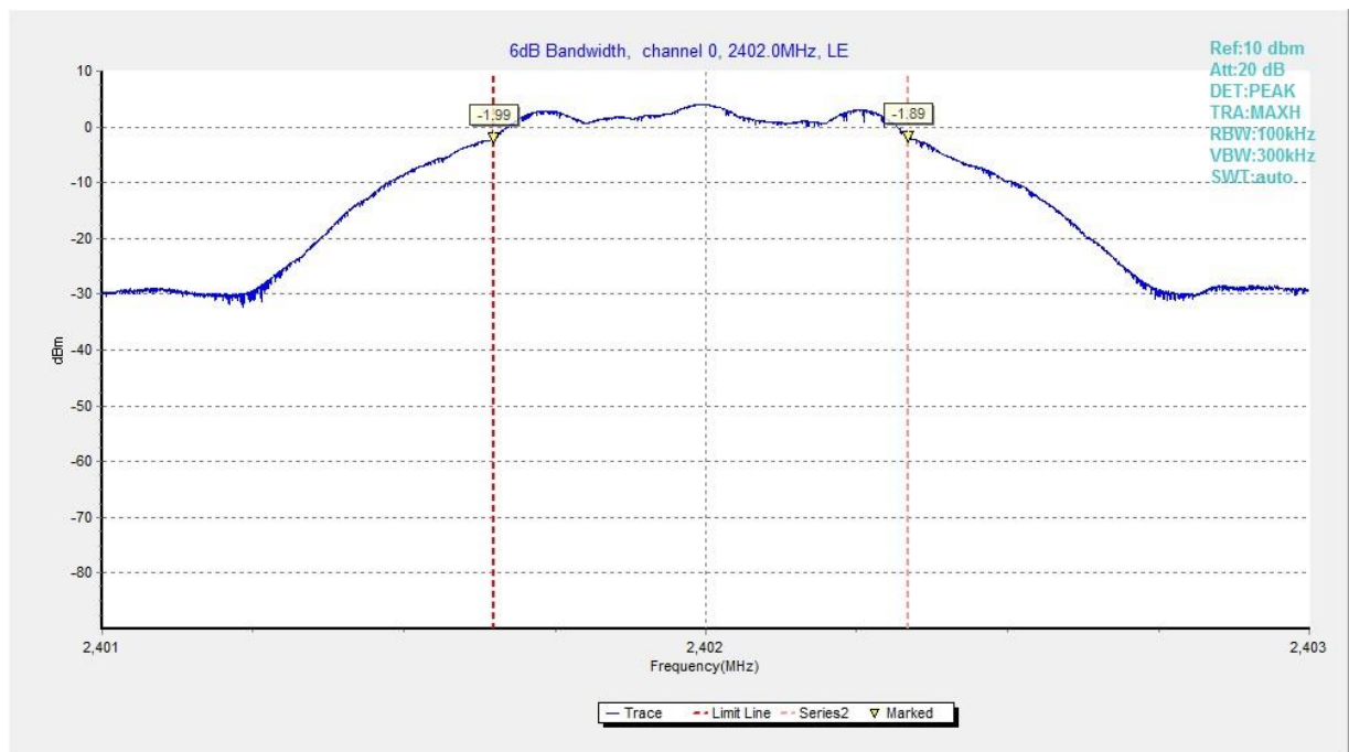
Fig.4 6dB Bandwidth (Ch 0), LE 1M
