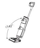
Do not recline the appliance more than 142° to protect against water leakage.
