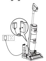
To charge the appliance, place the appliance on the charging base and plug the adaptor into a power outlet.
