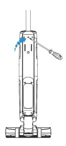
In the event that the product must be returned, please disassemble the handle. Press the spring to release the handle with a tool (like a screwdriver) and lift the released handle from the appliance.
