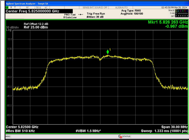
IEEE 802.11ac_Channel 165_20MHz_Antenna 0
