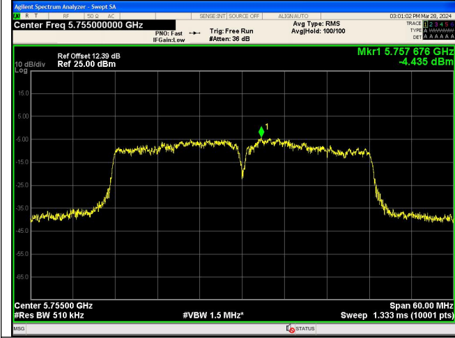
IEEE 802.11n Channel 151_40MHz_Antenna 0
