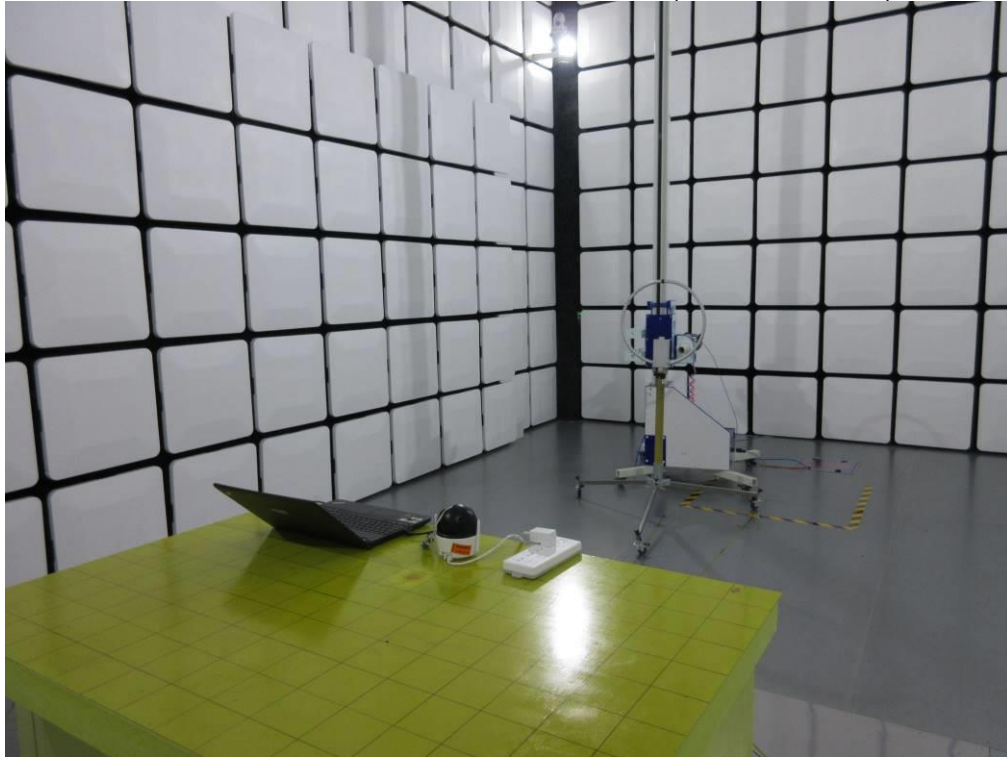
RADIATED RF MEASUREMENT SETUP (30MHz ~ 1 GHz)
