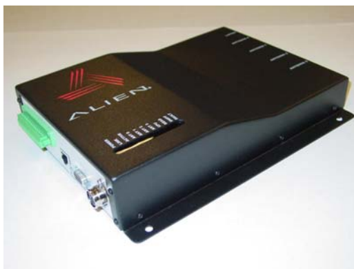
Figure 21 - View of the Reader showing mounting holes
