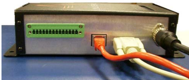
Figure 8 - RS-232 and Power Connections
