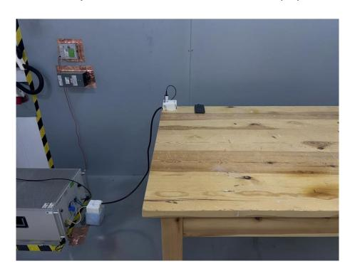
Set-up for Radiated Emission (RE), Below 1GHz
