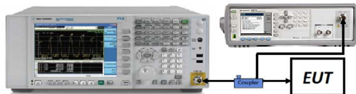
Figure 7-3. Test Instrument & Measurement Setup
