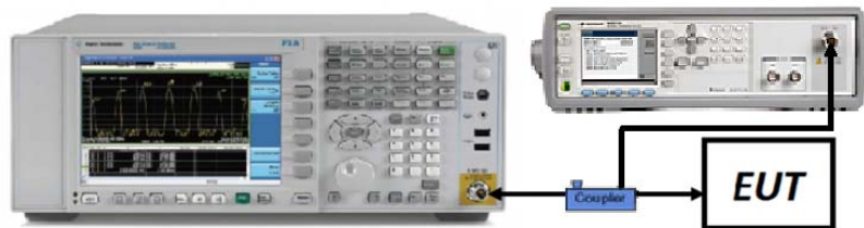
Figure 7-2. Test Instrument & Measurement Setup
