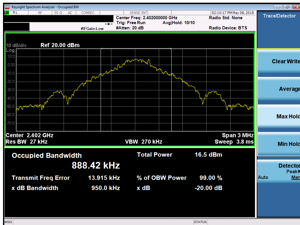
Plot 7-1. 20dB Bandwidth Plot (Bluetooth, 1Mbps – Ch. 0)
