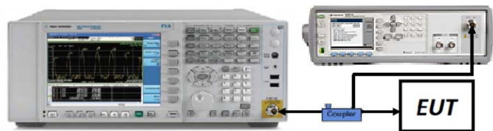
Figure 7-6. Test Instrument & Measurement Setup
