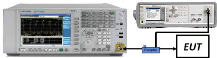
Figure 7-4. Test Instrument & Measurement Setup
