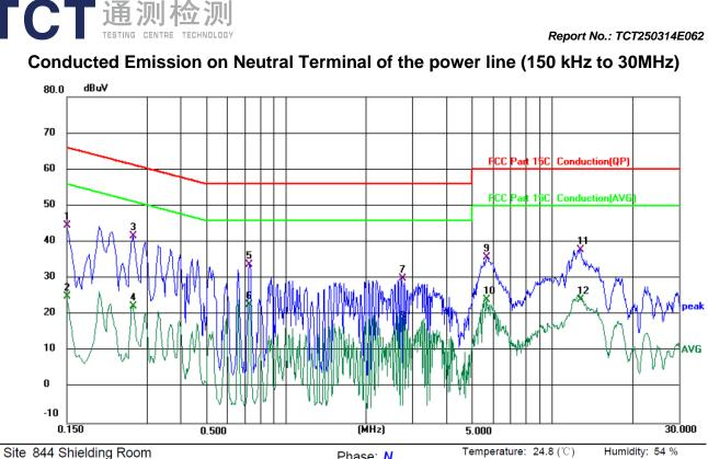
Limit: FCC Part 15C Conduction(QP)
