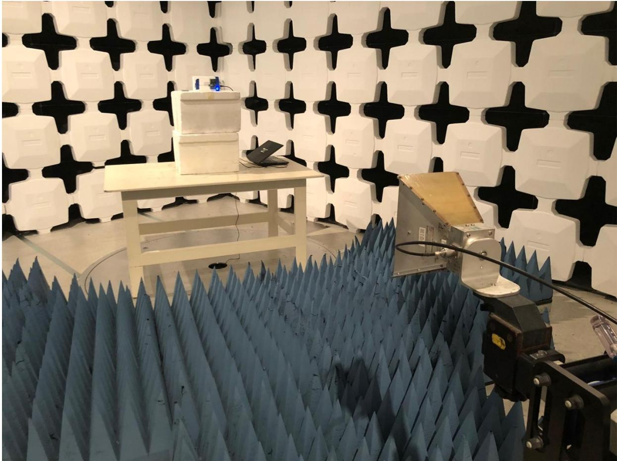
**Figure 4. Intentional Radiator, Radiated Emissions**
