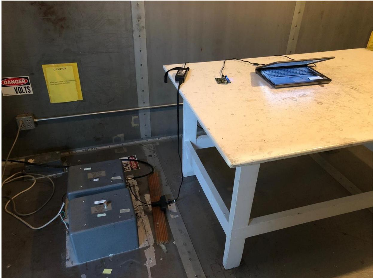
**Figure 5. Power Line Conducted Emissions**
