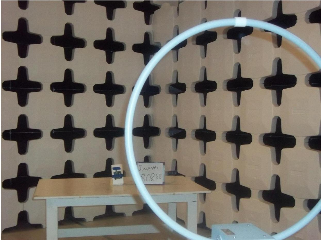
**Figure 1. Radiated Emissions Test Configuration (Below 30 MHz)**
