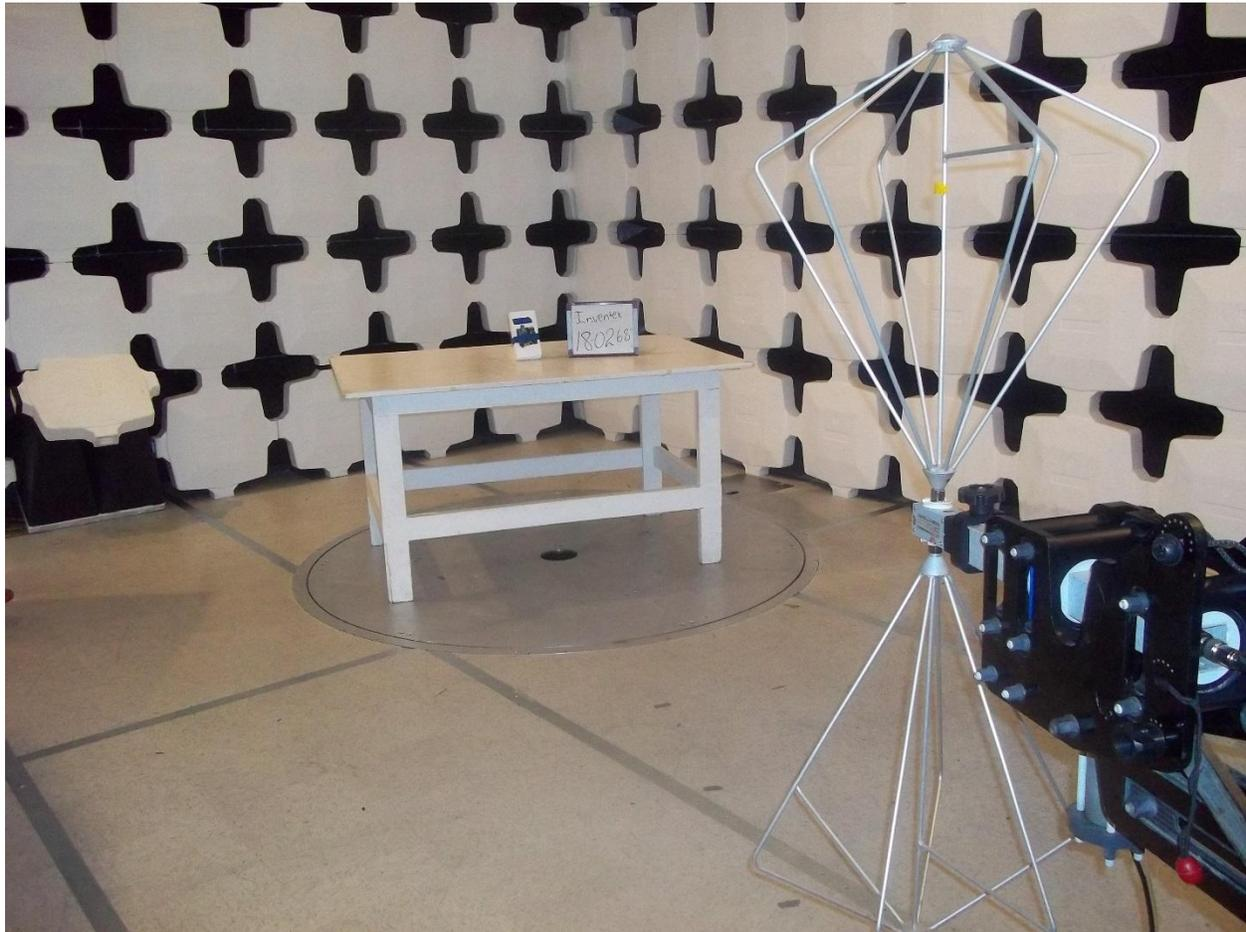
**Figure 2. Radiated Emissions Test Configuration (30-200 MHz)**
