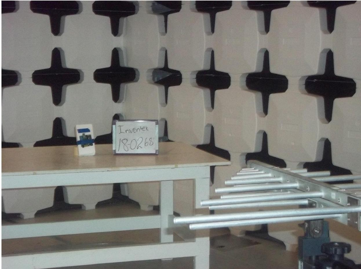
**Figure 3. Radiated Emissions Test Configuration (200 MHz to 1 GHz)**
