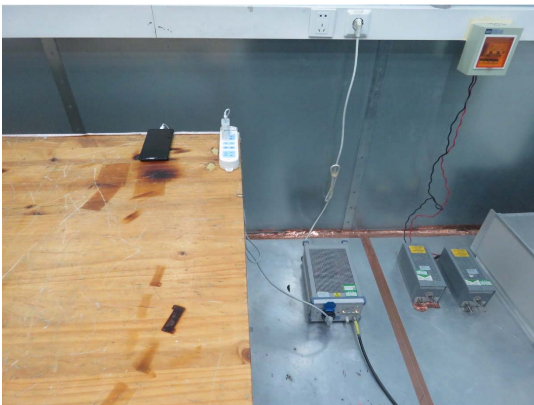
Picture 2 Conducted Emission Test Setup
