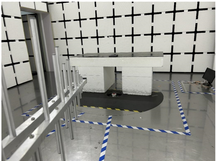
Radiation Emission Test Setup (30MHz to 1GHz)
