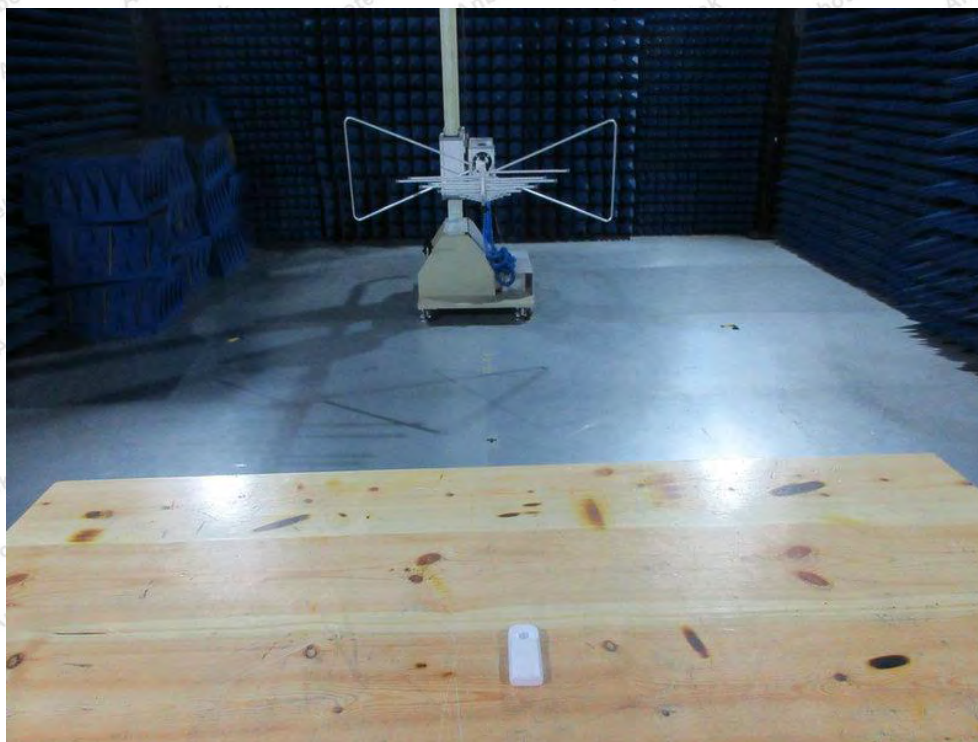
Photo of Radiation Emission Test
