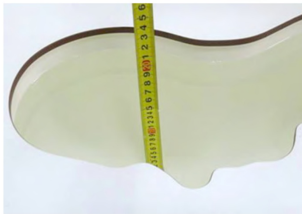
Liquid depth in the head phantom (835MHz)
