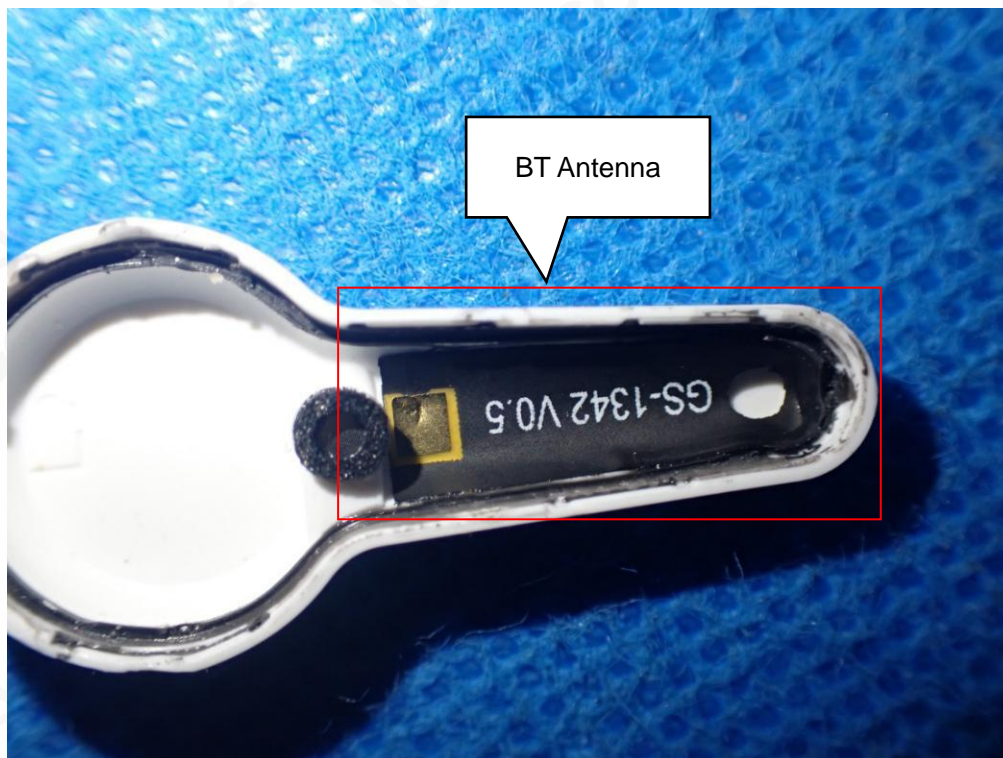
INTERNAL VIEW-1 OF EUT(Right earphone)
