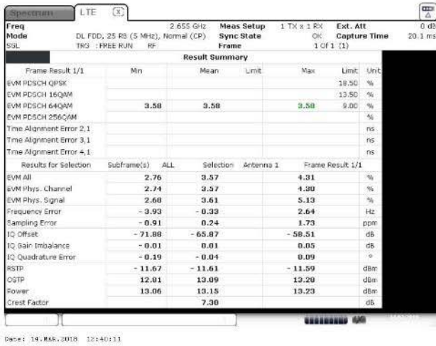
Figure 10. I/Q constellation table with I/Q error – 64QAM (2655 MHz) (5 MHz Channel BW)
