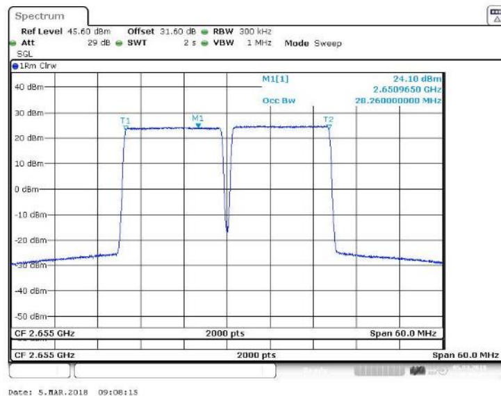
Figure 40 Occupied Bandwidth – 256QAM (2647.5 MHz, 2662.5 MHz) (2 X 15 MHz Channel BW)
