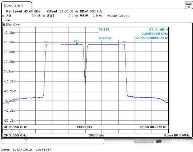
Figure 41 Occupied Bandwidth – QPSK (2645 MHz, 2665 MHz) (2 X 20 MHz Channel BW)
