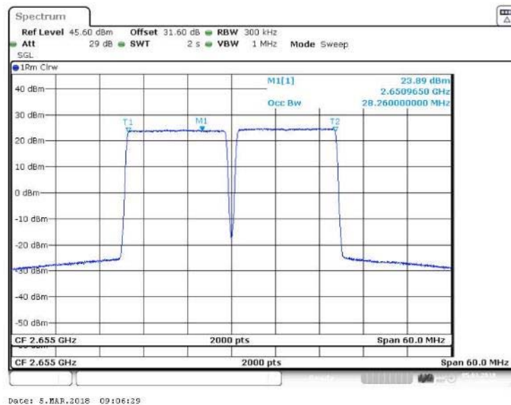
Figure 39 Occupied Bandwidth – 64QAM (2647.5 MHz, 2662.5 MHz) (2 X 15 MHz Channel BW)
