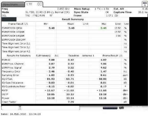
Figure 6. I/Q constellation table with I/Q error – QPSK (2655 MHz) (5 MHz Channel BW)
