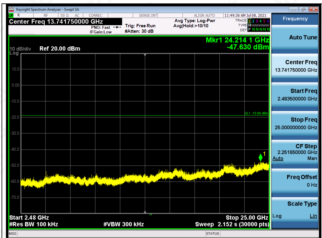
Test_Graph_LE1M_ANT1_2402_1Mbps_Higher Band Emissions
