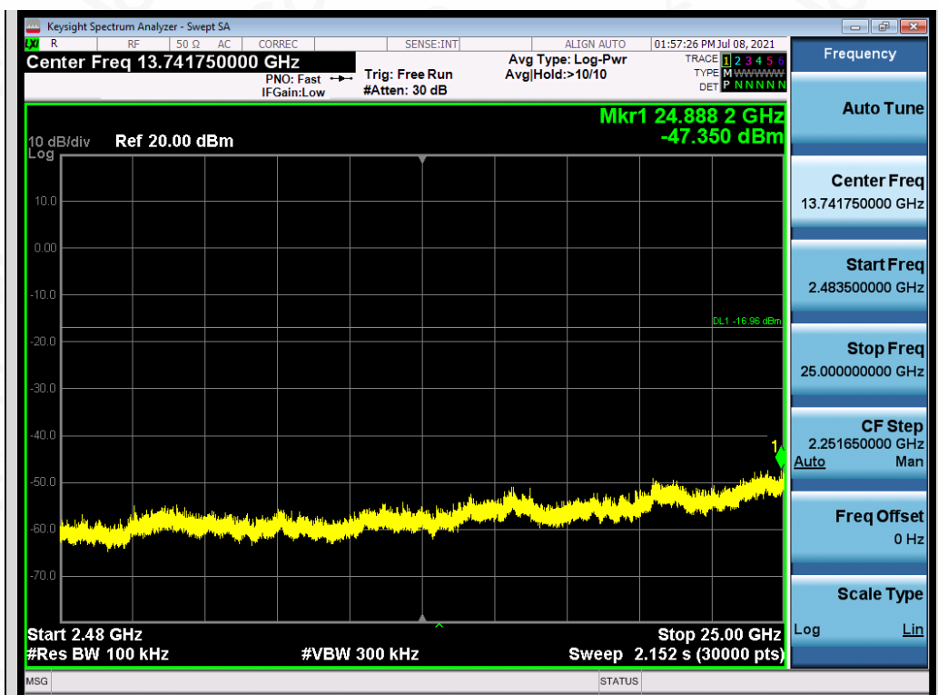
Test_Graph_LE2M_ANT1_2440_2Mbps_Higher Band Emissions
