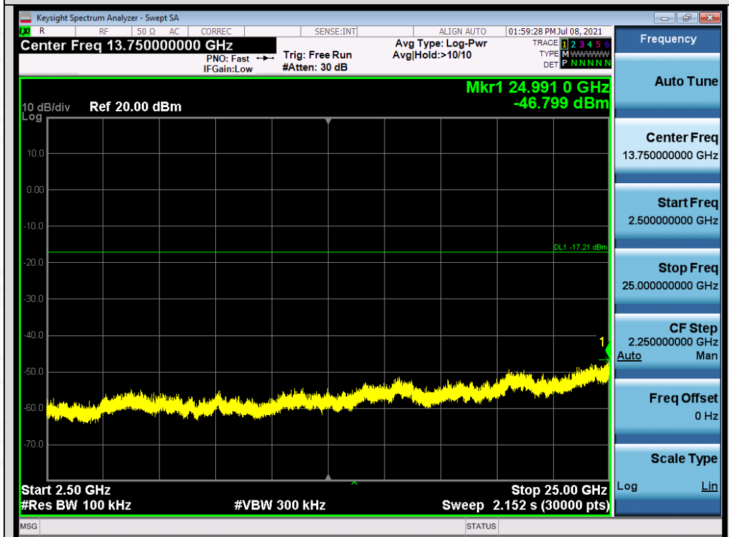
Test_Graph_LE2M_ANT1_2480_2Mbps_Higher Band Emissions
