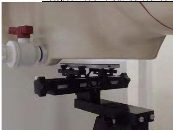
Fig.9 EUT Front side to flat phantom
