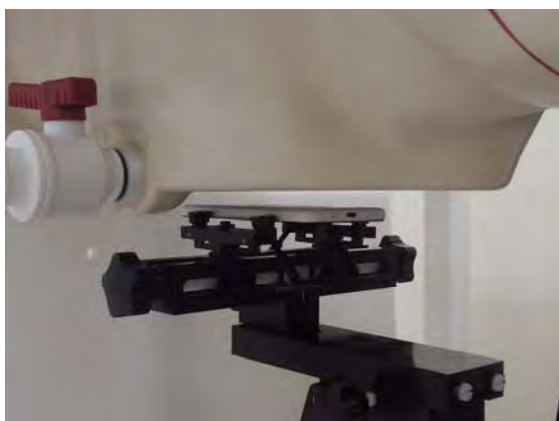
Fig.8 EUT Back side to flat phantom
