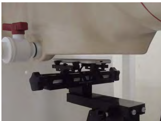
Fig.10 EUT Back side to flat phantom
