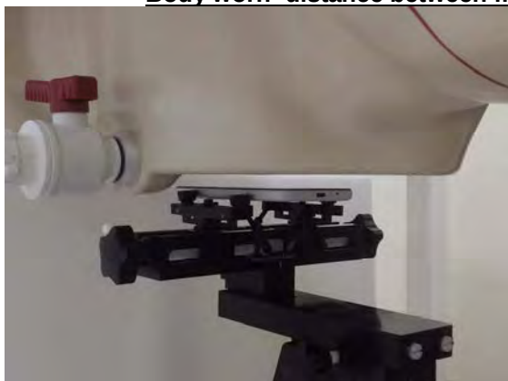
Fig.7 EUT Front side to flat phantom
