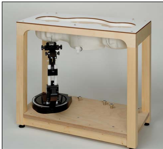
Figure 12: Specific anthropomorphic mannequin twin phantom
