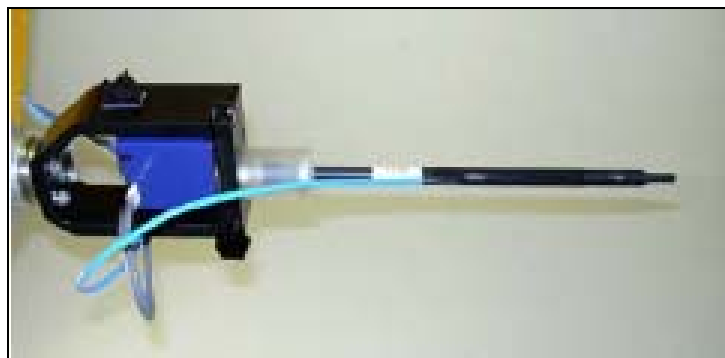
Figure 11: Electric field probe
