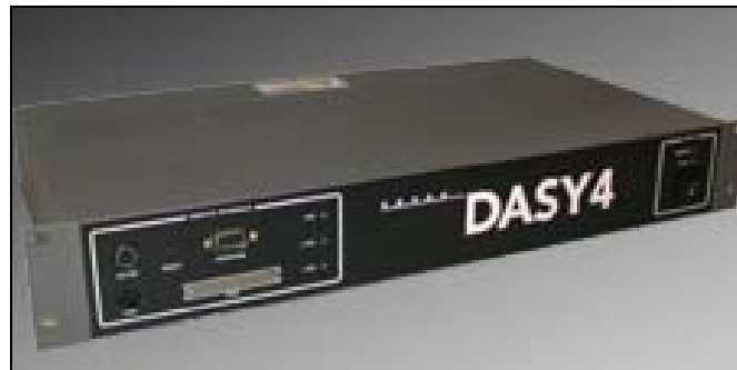
Figure 10: DASY4 measurement server
