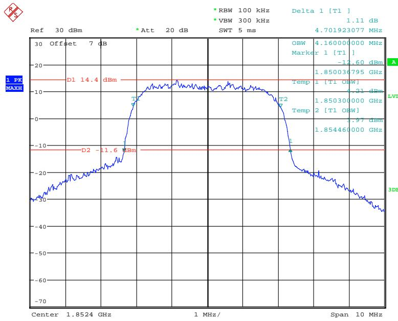
**26 dB Emissions & 99% Occupied Bandwidth for HSUPA (BPSK) Mode, Middle Channel**
