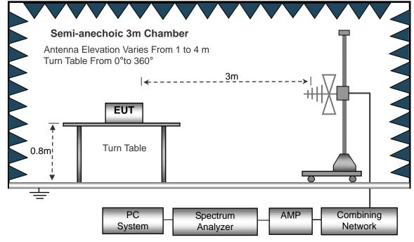
(C) Radiated Emission Test-Up Frequency Above 1GHz
