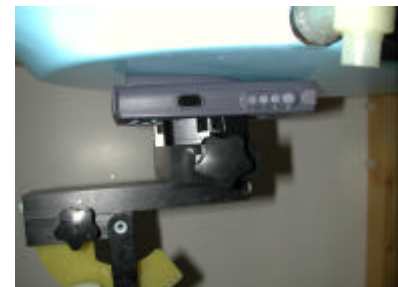
Figure 18. Body SAR Test Setup
