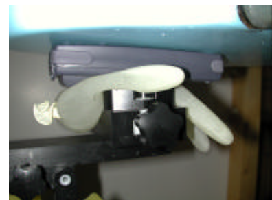
Figure 19. Hand SAR Test Setup
