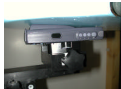
Figure 17. Body SAR Test Setup
