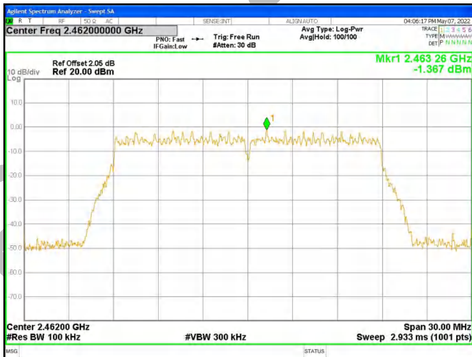
Band Edge NVNT n20 2462MHz Ant1 Emission
