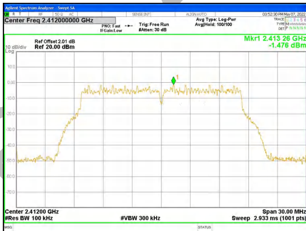
Band Edge NVNT g 2412MHz Ant1 Emission
