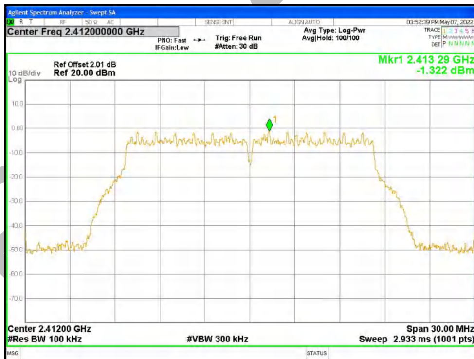
Tx. Spurious NVNT g 2412MHz Ant1 Emission
