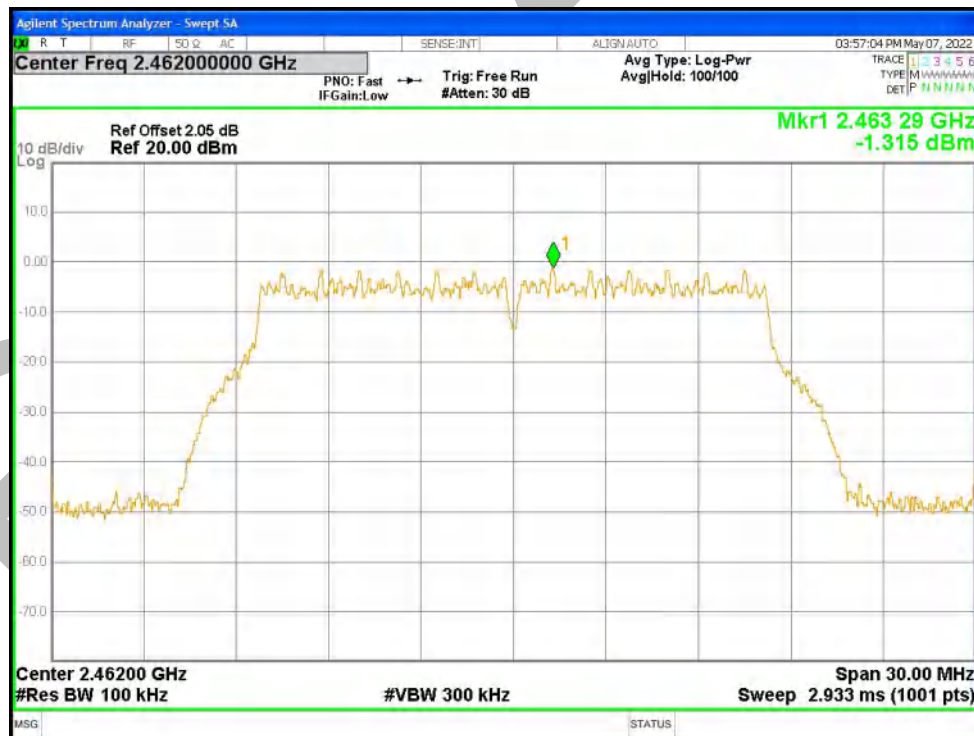
Tx. Spurious NVNT g 2462MHz Ant1 Emission
