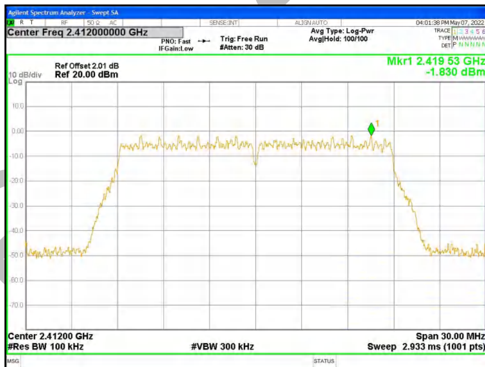
Tx. Spurious NVNT n20 2412MHz Ant1 Emission
