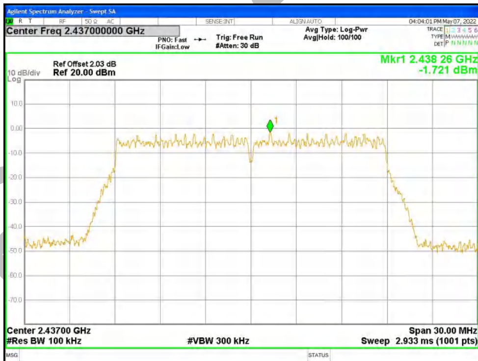
Tx. Spurious NVNT n20 2437MHz Ant1 Emission
