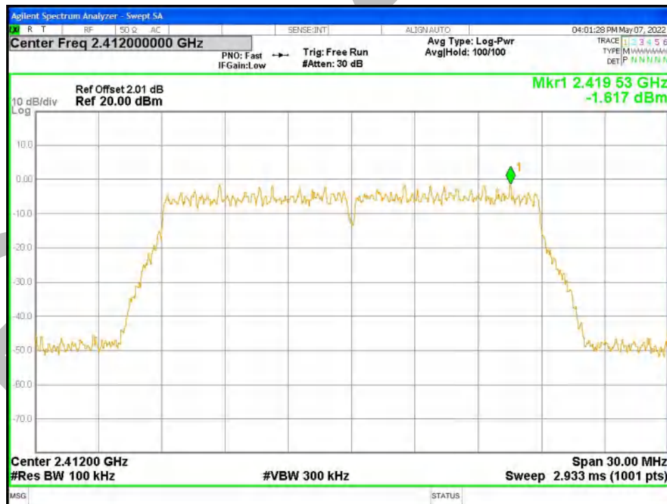
Band Edge NVNT n20 2412MHz Ant1 Emission
