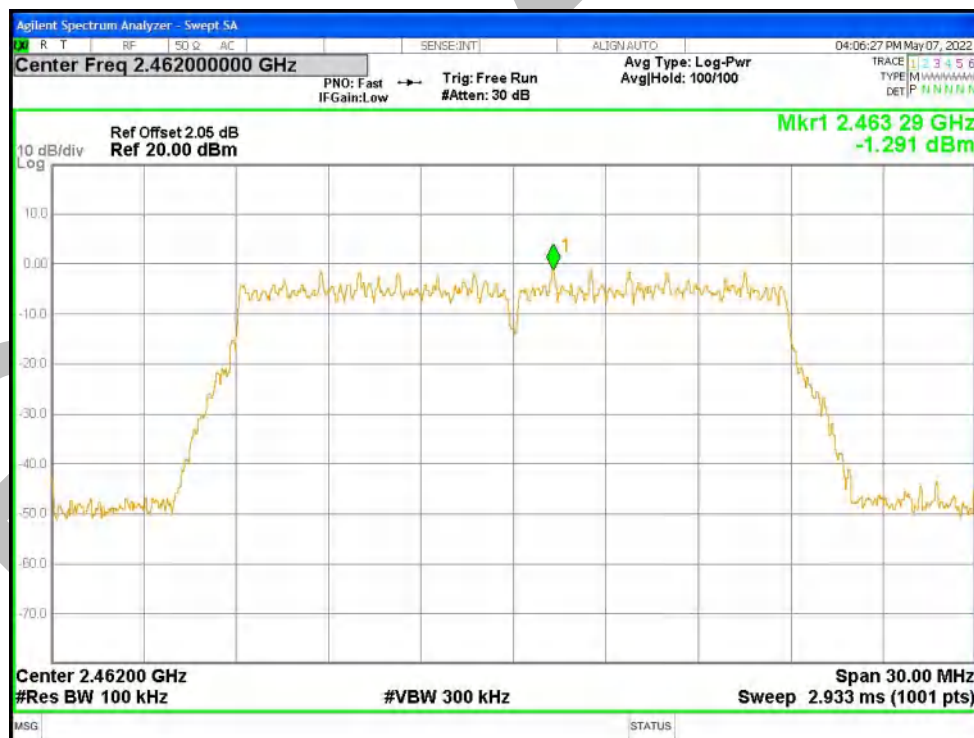
Tx. Spurious NVNT n20 2462MHz Ant1 Emission
