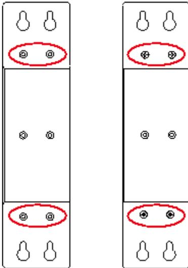
3. Remove the screws (packaged with the wall mounting plate), fix the screws in the mounting position with a screwdriver, and then pull down the device to make the device in a stable state, as shown in the figure below.
