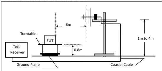
(c) For radiated emissions above 1000MHz
