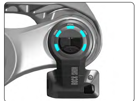
Rear Shock Low Speed Compression Damping (LSC) Setting - Cyan
